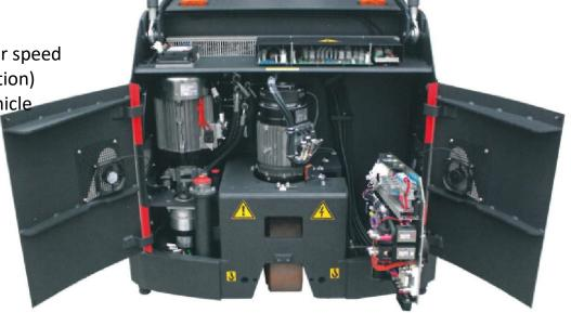
Motor compartment protected by strong steel maintenance doors.
