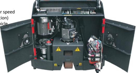
Motor compartment protected by strong steel maintenance doors.
